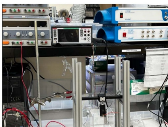
Figure 3. Experimental setup used for electromechanical and electrochemical characterization and corresponding schematic diagram. The measurements were conducted in wet conditions (in deionized water) at a room temperature (21 °C); therefore, the effect of water loss may be neglected. The electrochemical impedance spectroscopy (EIS) measurements were conducted in a two-electrode configuration. Furthermore, the electrochemical measurement plots were obtained from EIS measurements at a frequency range of 10 KHz–1 Hz utilizing an AC perturbation of 10 mV.
