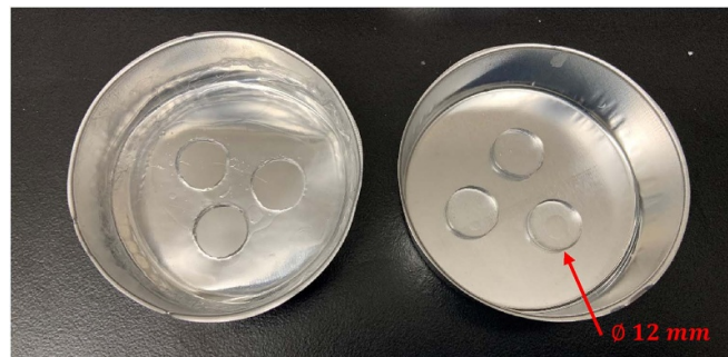
Figure 1. Sample preparation for mechanoelectrical experimentation by punching circular samples from a cured dish of PVC gel material ( left ) to help reduce edge effects and defects in the experimental samples ( right ).
