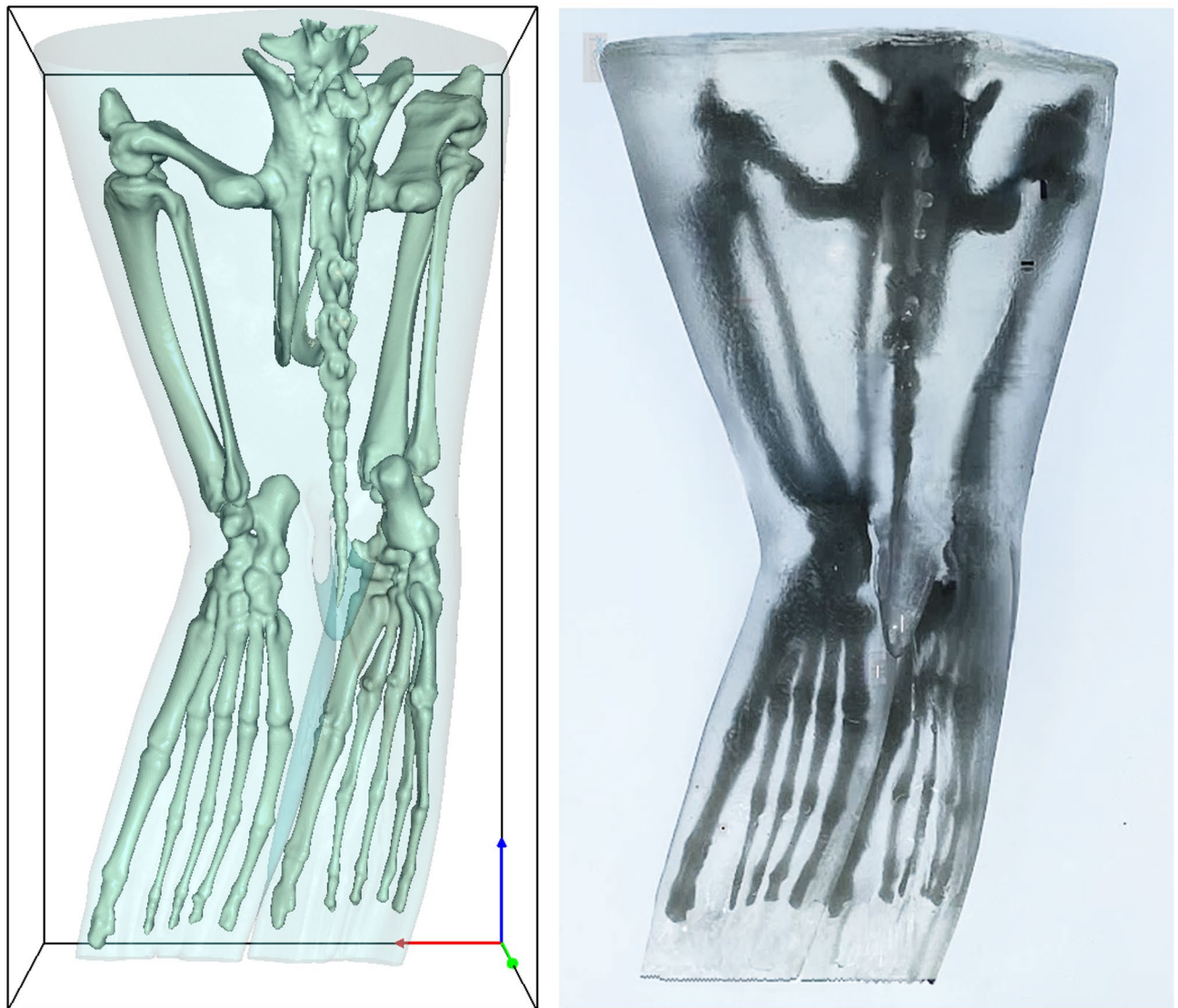
Fig. 9. Comparison of (left) original 3D render from Simpleware and (right) the final 20% scale fabricated phantom model. The printed model closely replicates internal skeletal features and anatomical contours with clear visual fidelity.
