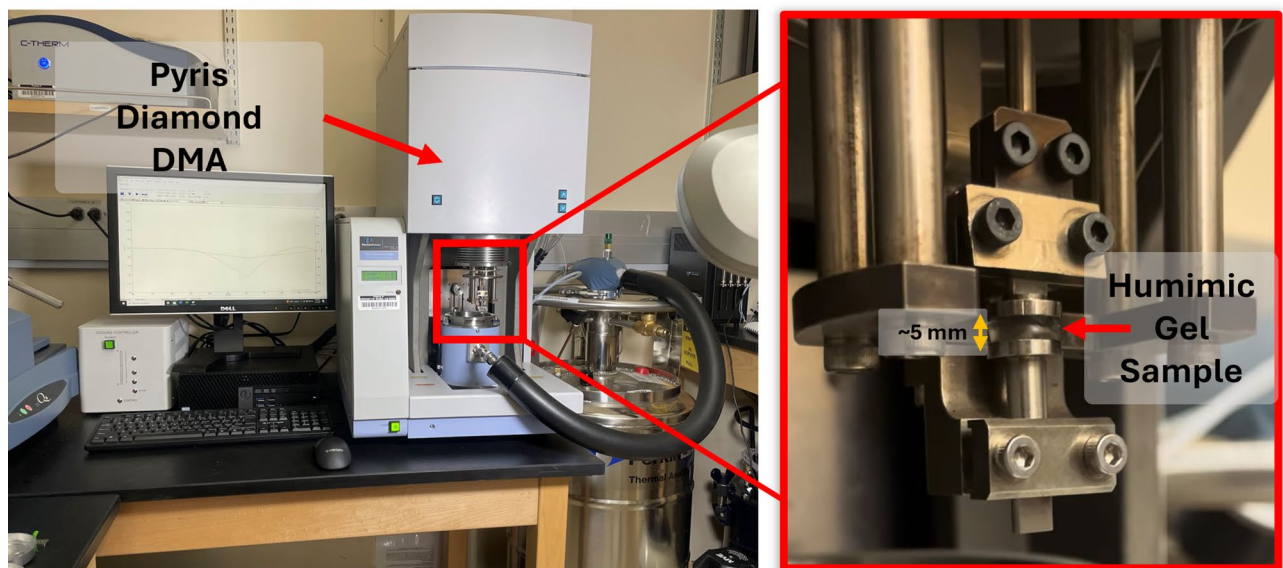
Fig. 5. Experimental setup for dynamic mechanical analysis (DMA) testing; (Left) PerkinElmer Pyris Diamond DMA system; (Right) Close-up of testing chamber with a Humimic gel sample mounted for compressive testing 19 .
