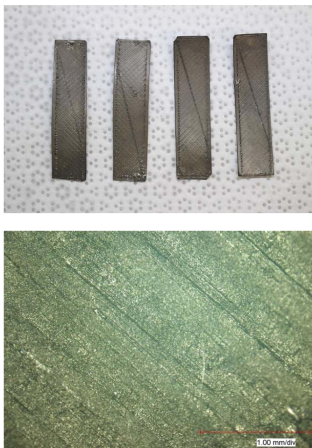
Figure 23. Four printed Aquivion IPMCs (Pr-Aq-IPMC) plated with platinum using the electroless plating process (top) and surface of one of the samples at 100x magnification (bottom).
